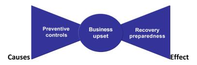
An bow-tie method shall be applied on risks perceived to be moderate or high in order to to identify possible proactive barriers to reduce or avoid incidents, or to reduce the consequences if the incident happen.
